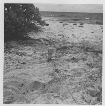
MICROBAROGRAPH "head" site on a lonely stretch of Ronjerik beach. Plastic tubes and fittings filter out the sound of the surf.
